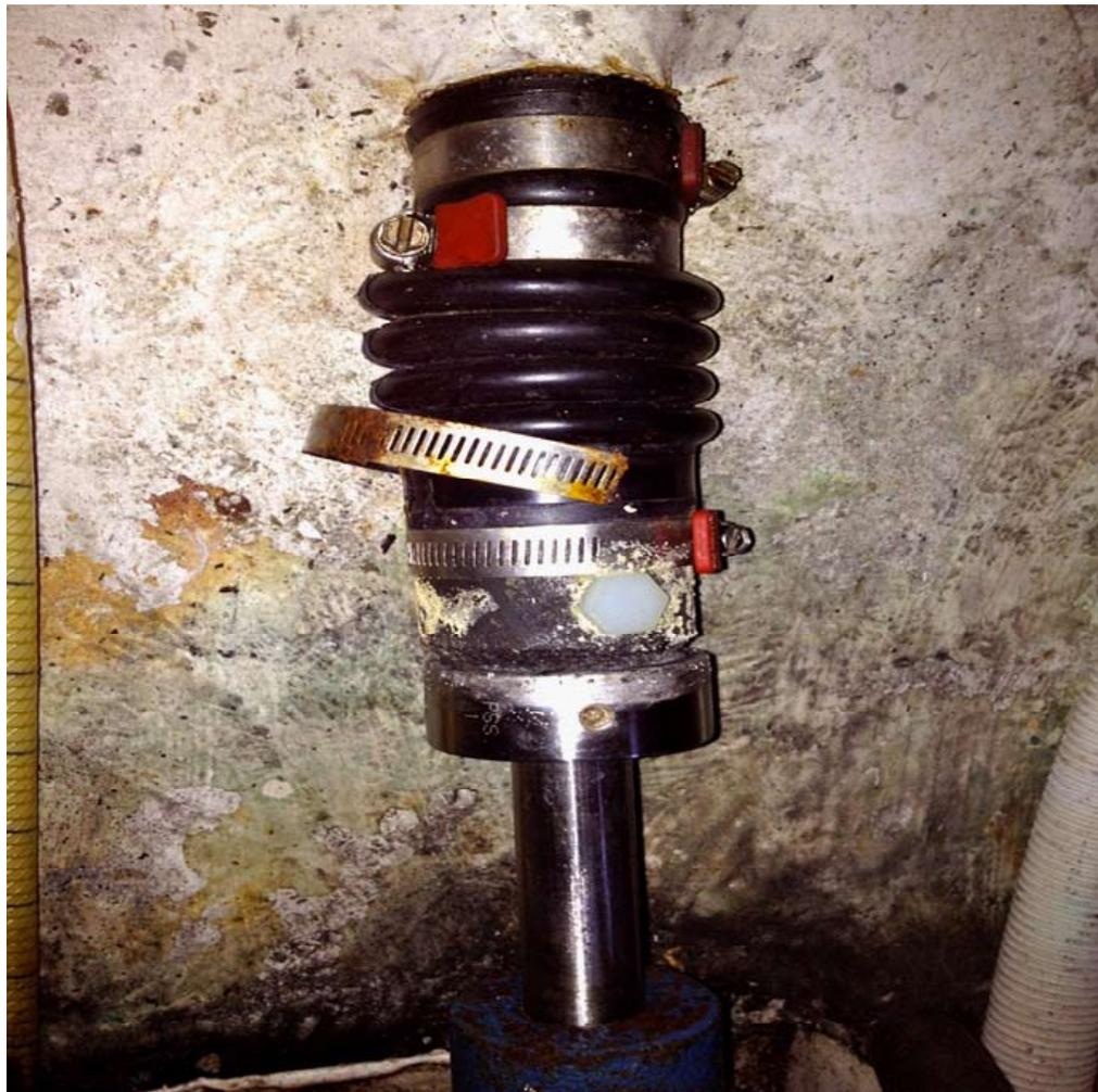
Yikes, I couldn't believe it...on my very own boat no less! Well, at least there were two clamps installed on each end. Interestingly, upon removal and visual inspection, the three remaining clamps were all seemingly in perfect condition.
