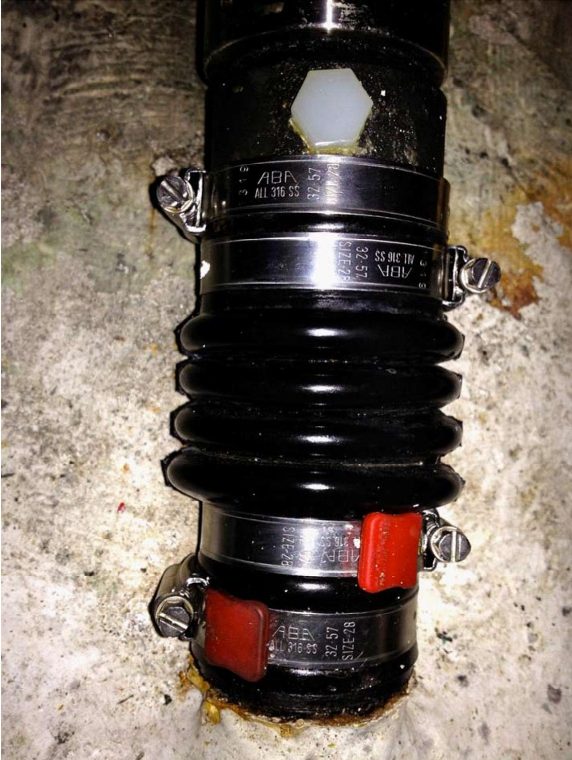
It might be difficult to make out from the photo but the new clamps are size 28, 316 stainless ABA worm-gear clamps as top rated by Practical Sailor. According to their test results these should last a long time...but don't worry, I'll be checking them frequently...don't want any more surprises like that again!
